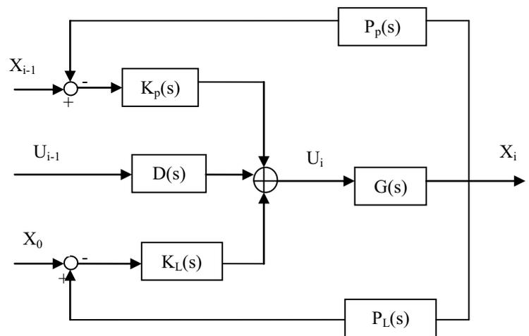
Fig. 2 Block Diagram of CACC controller
