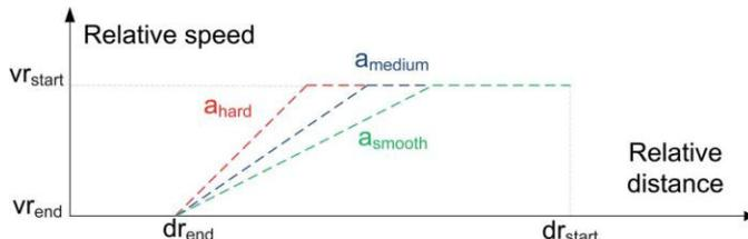
Fig.3 Gap closing controller operation
