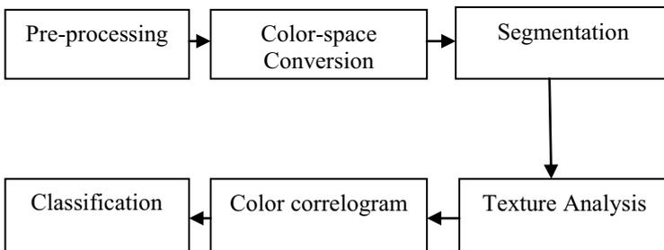
Figure 1:-Block diagram of proposed method
