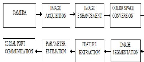
Figure 2: Block diagram of video signal processing
